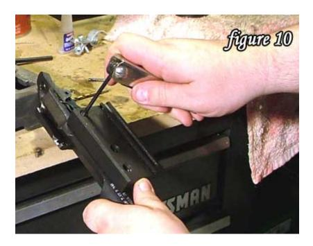
Next, I tightened the three screws. I did not use Loctite at this point yet because I wanted to make any adjustments needed at a later time.
