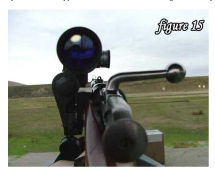
I took a leather cheek pad to install on the stock if I could not get a proper cheek weld. Unlike the Mauser project I completed with the same scope I found the Mosin Nagant stock provided a very adequate weld and the leather cheek pad was not necessary for me. This may be different for you. I guess I finally benefit from having chubby cheeks. Figure 15 shows how the new bolt handle easily clears the scope scope.
