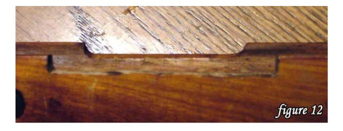
I used a rotary tool cutting disc and cut the wood out a little bit at a time until the mount fit snuggly. Figure 12 shows the amount of wood I removed.
