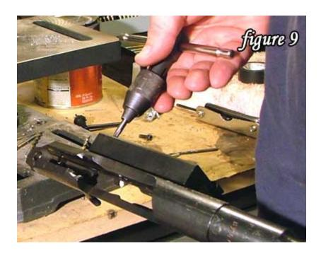
The 10-32 tap bit is what you use to cut threads in the receiver's drilled holes. You will have to purchase a tap handle similar to the one shown in figure 9. The prices of a tap handle ranges from \$5 and up depending on the quality. Oddly enough I have found the inexpensive \$5 handle to work best for me.
