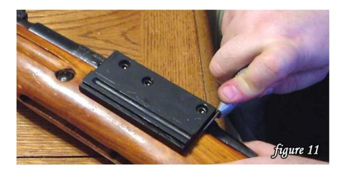
I installed the action into the stock and found I would need to inlet a small amount of wood for the mount to fit properly. I marked off the sides with a cutting blade.
