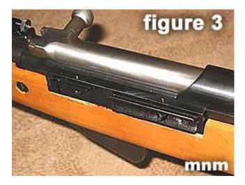
I drilled and tapped two holes for the mounting plate. The holes are very large in the side plate, I had to drill and tap using a 10-24 tap. Once the side plate is mounted to the receiver, I next had to remove some wood from the stock.
