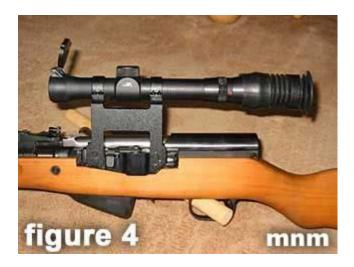
The finished rifle looks very Russian now. The scope mount easily comes off and makes cleaning and storing the rifle much easier. You can even take the scope off at the range. Just remount the scope, lock it down and it always returns to zero.
